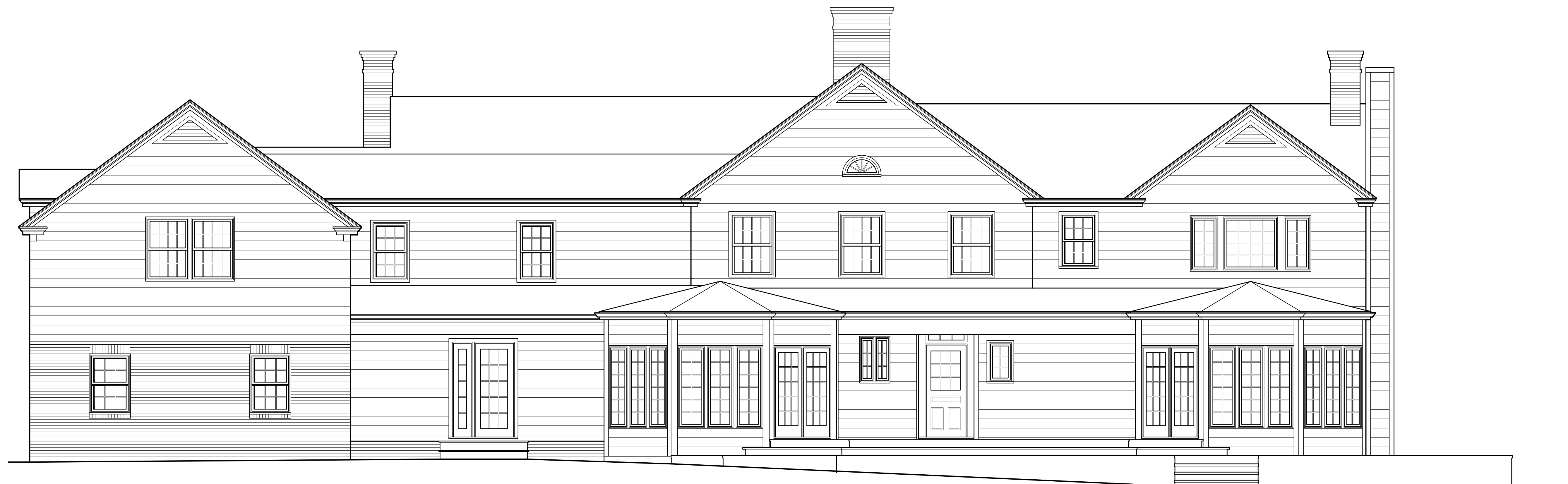
1 EXISTING REAR ELEVATION V-4 SCALE: 3/16" = 1'-0"
